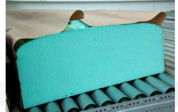
Production and testing of polyurethanes with CO<sub>2</sub>
