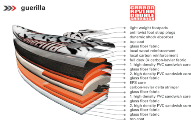
FIGURE 5 - Structure of a windsurf board [14]
