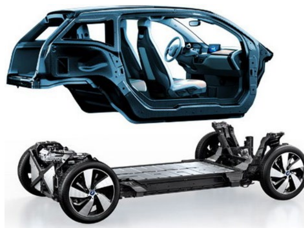
FIGURE 3 - BMW i3 CFRP life module (upper part) [12]
